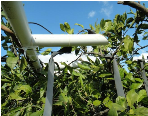
Figure 1. Photo of wetness sensors mounted on the upper citrus canopy at the Welgenvallen Experimental Farm, University of Stellenbosch between July and November, 2012.
