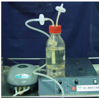
Figure 2. Two-in-One MPOB Simple Impeller (2-in-1 MoSLIM)
